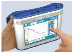
Dedicated logger – does not require a computer.
